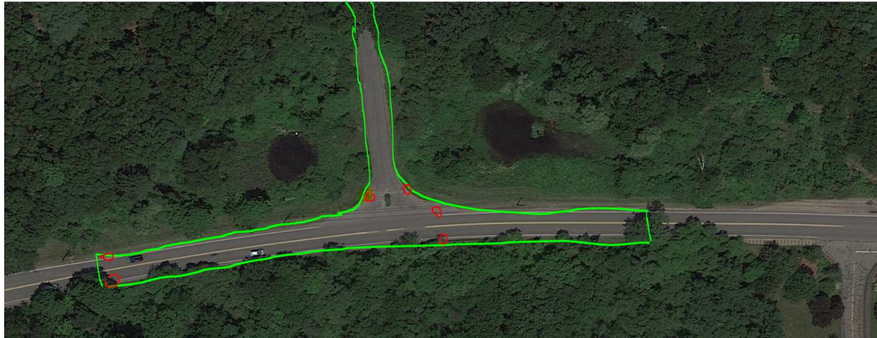
Figure 5. Alternative 2C drainage area from access road and Commonwealth Road (existing catch basins are circled in red)
