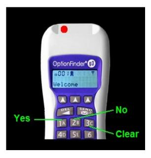
If you inadvertently turn your handset off by pushing the power button in its lower-right corner, its display will be blank; push the power button briefly to turn your handset back on. Pushing any of your handset's other buttons during the voting interval will not change your vote, but for peace of mind, your handset will encourage you to *Re-Vote*; push the 1 button for *Yes* or the 2 button for *No*.
