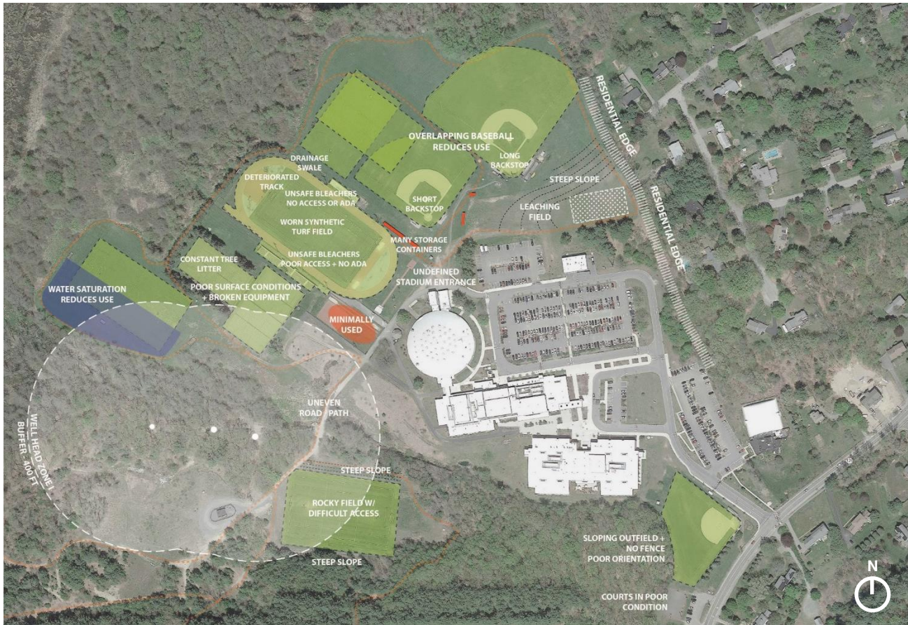
Figure 2: Summary of existing field conditions and limitations as well as well head zone 1 protection areas. Wetland resource areas form the much of the southern, western and northern perimeter of the property.
